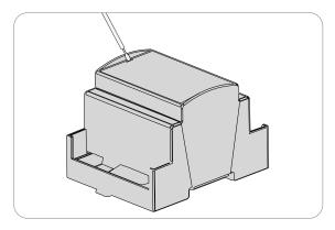
Insert the tip of a flat screwdriver (4.0 x 50 mm or similar) in the small opening on top of the driver.
